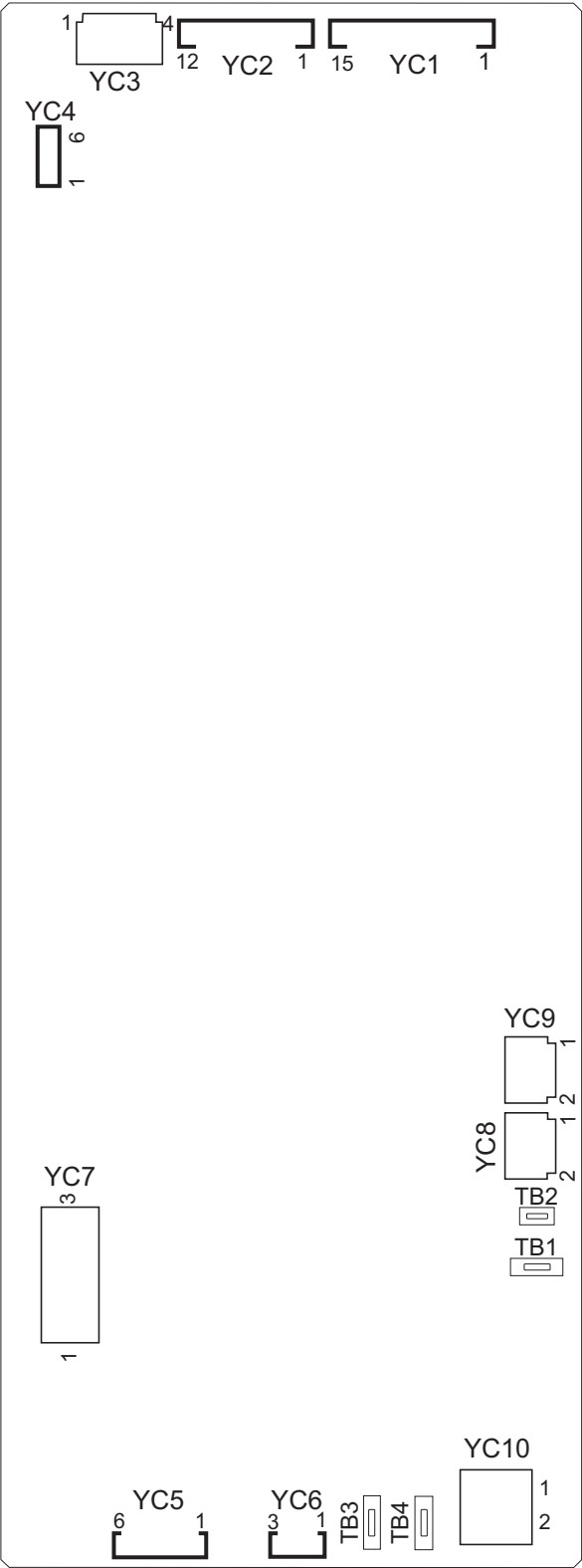
Figure 2-3-3 Main PWB silk-screen diagram
